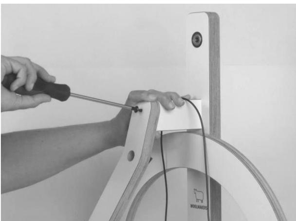
*Add the drive band to the assembly and screw the front post to the upper rail and base rail.*
